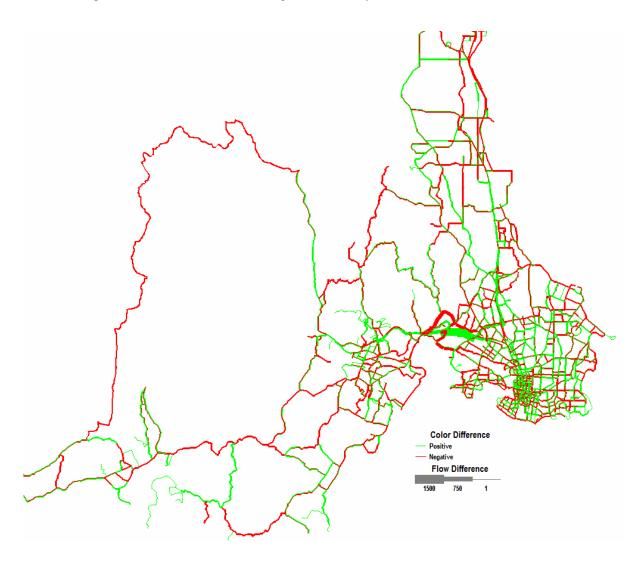
Figure 5: FW Flow Changes from Added Lanes at a Relative Gap of .001
