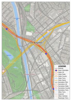
There are many reasons to have a GIS as part of a travel demand forecasting package. First, GIS makes it possible for planning models to be much more accurate. For example, network distances are based on the actual shape of the road network and a correct representation of highway interchanges.
